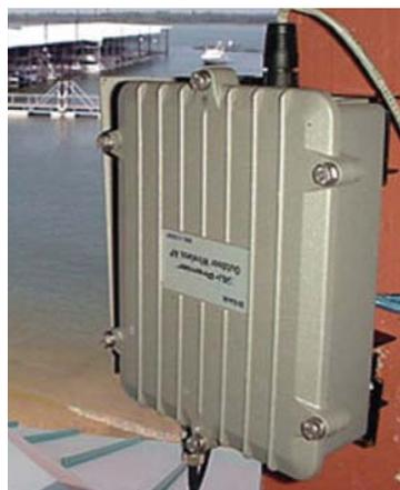
*The D-Link DWL-1700AP Outdoor Wireless Access Point is encased in a die-cast watertight housing and offers a wide-range of Enterprise level connectivity features.*
